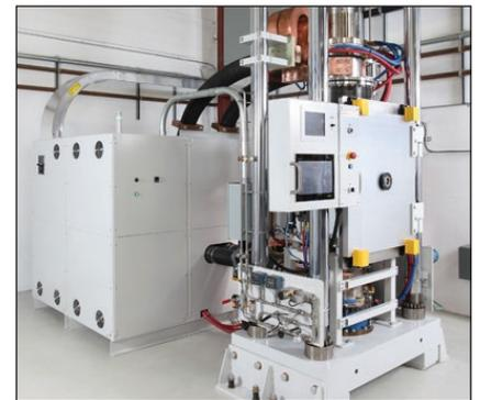
DCS 100 and 200: 100 and 200 tons force, and 30,000 and 50,000 amps
